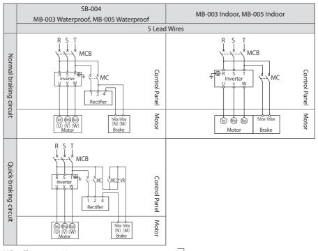
MC: Electromagnetic contactor
