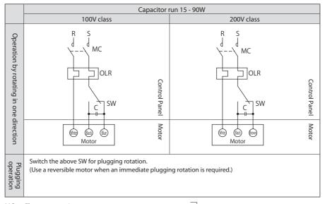
MC: Electromagnetic contactor
