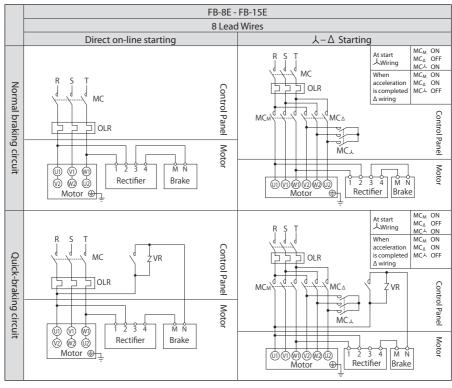
MC: Electromagnetic contactor
