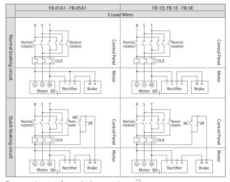
Electromagnetic contactor for normal and reverse rotation
