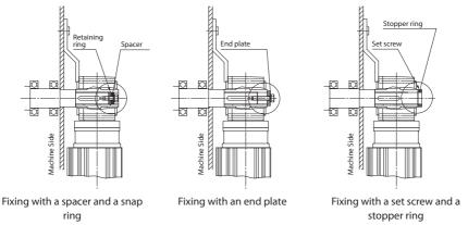
Figure 5-11 Method of Fixing In Which the Product Does Not Move in the Opposite Direction of the Machine
