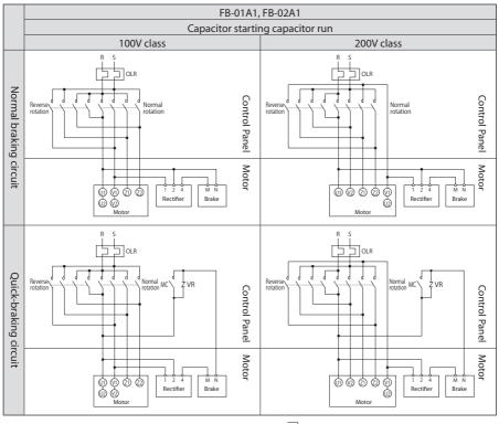
$\label{lem:contactor} \textbf{Electromagnetic contactor for normal and reverse rotation}$
