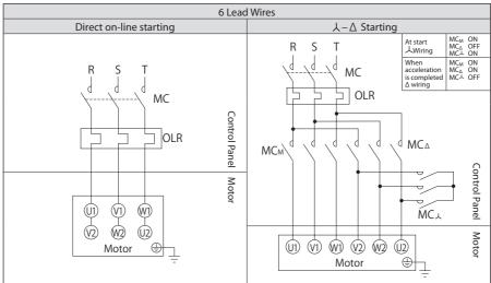
MC: Electromagnetic contactor
