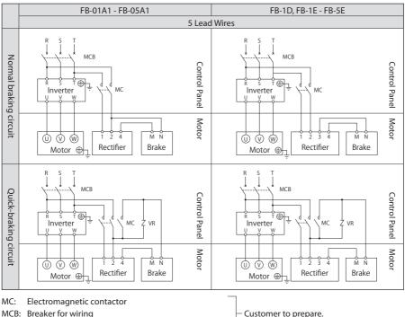
VR: Varistor (for protecting contact points, rectifier, etc.) Customer to prepare.
