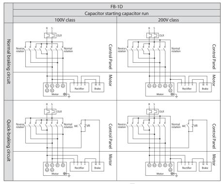
Electromagnetic contactor for normal and reverse rotation
