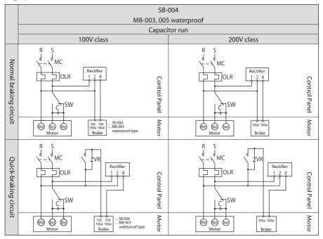
MC: Electromagnetic contactor
