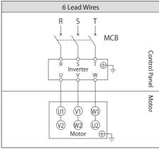
MCB: Breaker for wiring - Customer to prepare.
