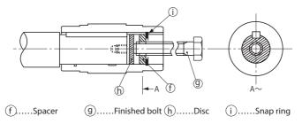
Figure 5-13 Removal Jig
