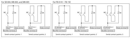
Note: 1. For inverter drives, connect to the R phase (power source side).
