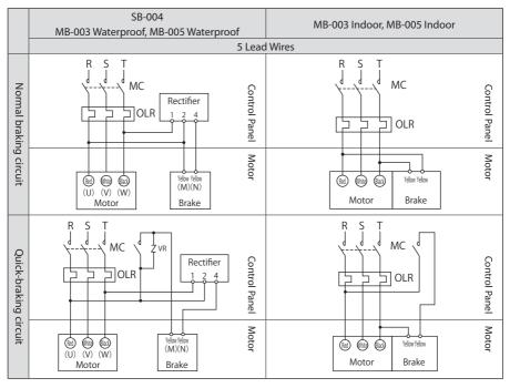
MC: Electromagnetic contactor
