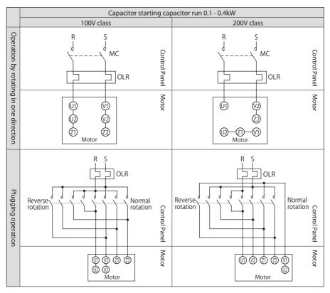
MC: Electromagnetic contactor
