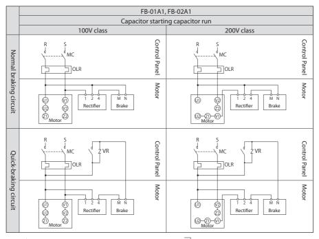
MC: Electromagnetic contactor
