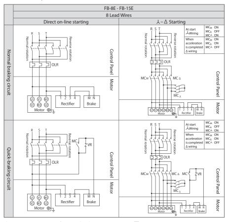
Electromagnetic contactor for normal and reverse rotation
