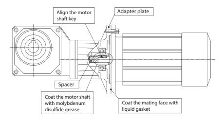
Figure 4-1 Assembly Diagram
