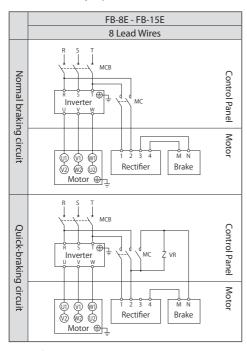
MC: Electromagnetic contactor
