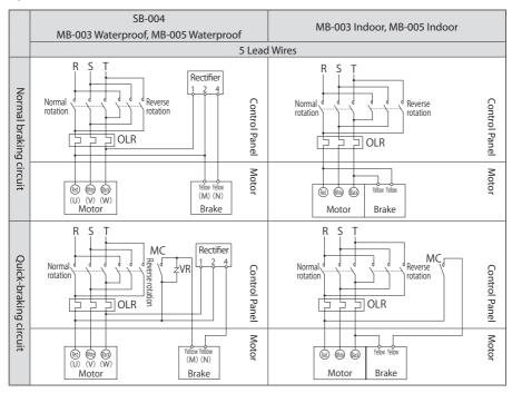
Electromagnetic contactor for normal and reverse rotation
